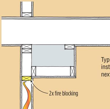
Typically, fire blocks are installed in the stud bays next to soffits.
